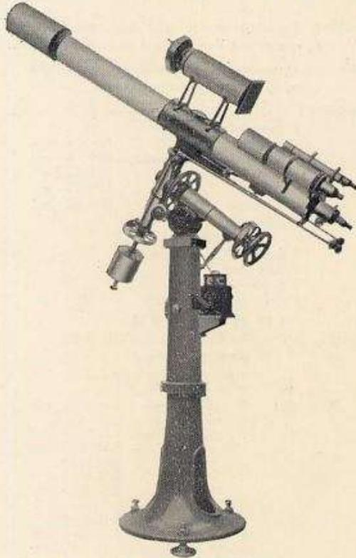
★ **Mounting** Equatorial mount, with R. A. and Decl. circles and slow motions on iron pillar stand.
